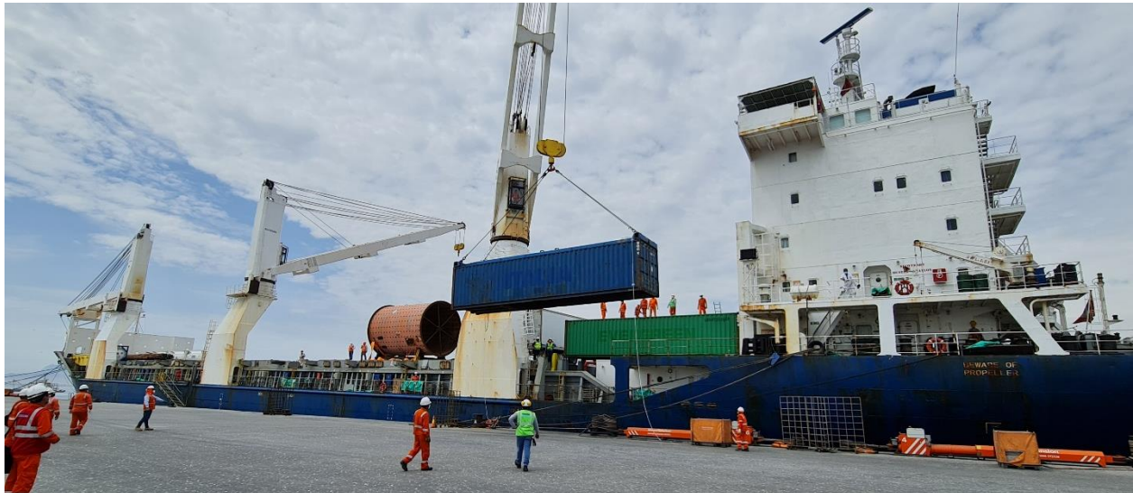
Figure 2. Major components of ball mill transportation in Salaverry, Peru
